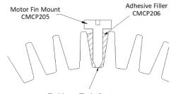
Fin Mount Tip In Contact With Motor Base
