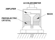
Accelerometers are inertial measurement devices that convert mechanical motion to an electrical signal. This signal is proportional to the vibration's acceleration using the piezoelectric principle. Inertial measurement devices measure motion relative to a mass. This follows Newton's Third Law of Motion: A body acting on another will result in an equal action on the first.
