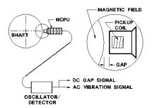
Eddy Probes are used on machines with Journal (Sleeve) type bearings. Where the measurement of motion between the Bearing and Shaft is critical.
