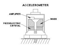
Accelerometers are a piezo-electronic (crystal) device. A pre-loaded crystal is charged with current and as the crystal is compressed or de-compressed by vibration an output proportional to g's (gravity) is provided. A "g" is equal to 9.80 meters/second<sup>2</sup> or one (1) standard earth gravity.
