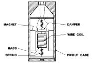
Velocity Transducers are normally used for Bearing Cap Vibration Monitoring (Case/Bearing Cap Absolute) on machines with rolling element bearings. They have the advantage of high outputs and the signal is read directly in velocity (in/sec or mm/sec).
