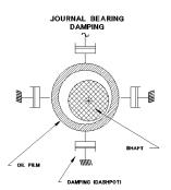
Journal or Sleeve Bearings are designed so that the oil film provides damping. The shaft is free to vibrate within the bearing. Due to the damping provided by the oil film very little of the shaft vibration is transmitted to the bearing cap. The oil film damping provides even higher levels of attenuation to higher frequencies.
