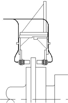
Perpendicular 90° Collars can be measured by either a single Eddy Probe transducer or by complimentary transducers mounted on either side of the collar. The size of the collar face available for the Probe viewing surface and the required measurement range will determine which method is best suited for the application.
