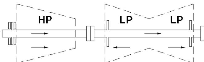
Differential Expansion on a turbine is the relative measurement of the rotor's axial thermal growth with respect to the case.
