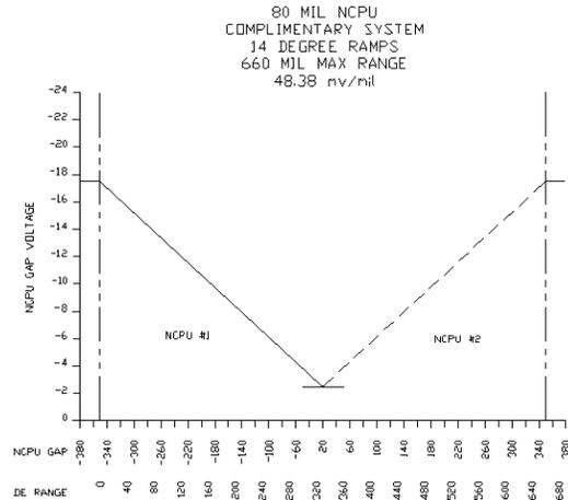
For this application, one the governor side pickup will be calibrated (adjusted or gapped) electrically, while the other will be calibrated mechanically while the turbine is in the cold condition.
