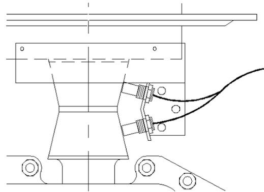
A Rotor Ramp installation can also be measured using either a single Eddy Probe transducer or by complimentary transducers configuration. The size of the Probe viewing surface and measurement range required will determine which method best suites the application.
