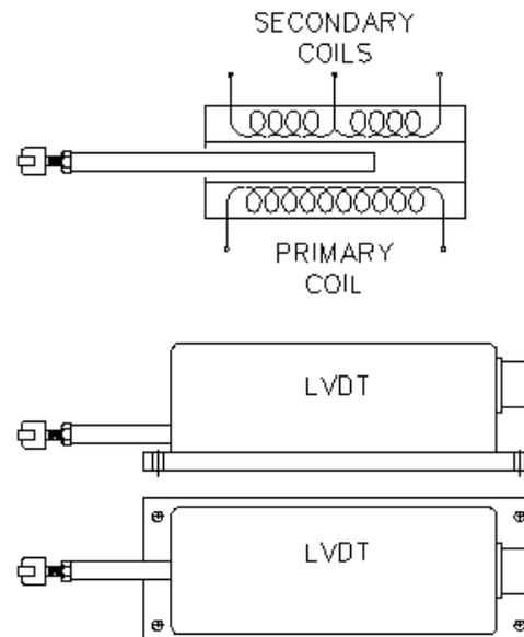
When the plunger is centered in its range the induced voltage of the two secondary coils is equal in magnitude, but opposite polarity. As the plunger moves to either side of the center position the voltage of one of the secondary coils increases while the other secondary coil experiences a decreased voltage. DC LVDT's differ from AC LVDT's in that they are manufactured with an internal carrier generator/signal-conditioning module and only require DC Power to operate.
