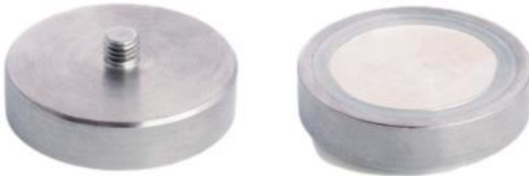
CMCP-MB03F Large Magnetic Base for flat surfaces, 110 Lbs Pull Strength, 1.40" diameter, 1/4"-28 Stud
