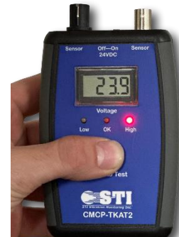
Shown Above: CMCP-TKAT2 Shows Open Circuit
