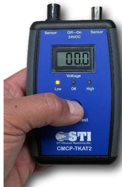
Shown Above: CMCP-TKAT2 shows Short Circuit
