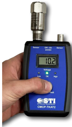
Shown above: CMCP-TKAT2 with Accelerometer attached
