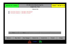
**4. Alarm List:** The System will list all active alarms on the Alarm List along with Tag Name, Date and Time, Type of Alarm. Only Active Alarms are shown.
