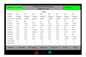
**6. Setup:** The Setup screen is used to turn channels off and on, enter tag identification, enter meter scales and activate and enter alarm set points. Relays assignments are also completed on this screen. By pressing "Setup" again the Company Information Screen is reached to change Header Name and Location along with date and time.
