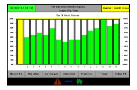
2. Alert Bar Graph: The Alert Bar Graph is a graphical representation of each channels % of its Alert Set Point. The Alert Set Point is at the top of the Bar Graph. The Current Value Bar is the percentage of that set point.
