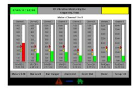
**1. Meter Display:** Unlike older monitoring systems the meters are fully configurable. Green, Yellow and Red Current Value Bars represent alarm status. Setpoints are displayed on screen in color. 8 Meters are shown per screen.
