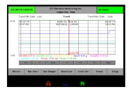
7. Trends: Up to 16 Trend Lines can be shown on a single screen. Trending does not need to be enabled if you are using a plant Historian. Standard setup is 1 minute intervals for a period of 2 weeks. The system will store a total of 10 two week files for a total of 20 weeks of data. Trend data is also available in .csv file format via connecting to internal web server or ftp. Optionally Trend intervals and length may be adjusted to suit your needs.
