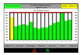
**3. Danger Bar Graph:** The Alert Bar Graph is a graphical representation of each channels % of its Danger Set Point. The Danger Set Point is at the top of the Bar Graph. The Current Value Bar is the percentage of that set point. The Current Value Bar will be Yellow if it has exceeded the Alert Set Point.
