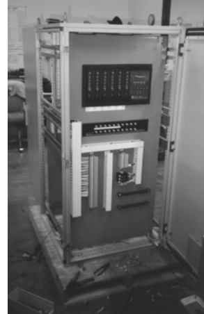
M800A Monitor, BNC Panel, Terminals, Power Distribution, Low Noise Configuration, Ground Bars, integrated into Modular Custom Cabinet for ARAMCO by STI.
