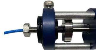
4. Rotate the micrometer in 0.005" (English) increments using the patented QuickClick adapter. The adapter is indexed allowing for quick and repeatable adjustments.
