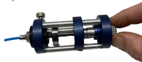
5. Record the DC voltage output from the proximity probe with a Digital RMS Voltmeter and record enter the data into the Probe Calibration Curve Generator provided with the calibrator in Microsoft Excel format (see graph on next page).
