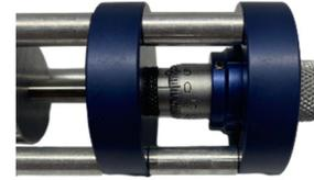
2. Insert the Proximity Probe into the correct size Collet. Collets are provided for 1/4", 3/8", M8 and M10 Probes.
