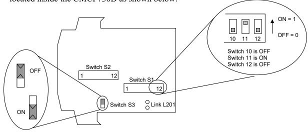
Switch S1, S2 and Link L201 configure the input type and range, and switch S3 configures the output type. The switch settings are explained in the next few pages. The diagrams refer to switch positions 0 and 1, with 0 being OFF and 1 being ON. This is illustrated in the picture above.
